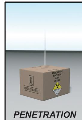
Penetration test by dropping a 13-pound, 1.25-inch diameter bar vertically onto the package from a height of 3.3 feet (1 meter).
