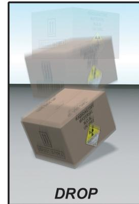
Free drop test onto a flat, hard surface. Drop distance varies based on weight of package (see below).
