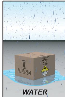
Water spray for 1 hour to simulate rainfall of 2 inches per hour.
