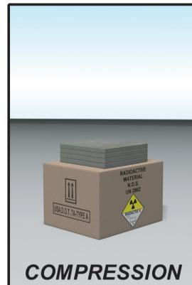
Stacking test of at least 5 times the weight of the package. This test is conducted for at least 24 hours.
