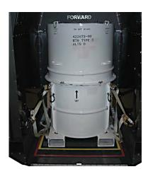
Type B packages must pass strict testing governed by both the DOT and NRC. They are used to transport material with high levels of radioactivity, provide radiation shielding, and can range in size from small to several tons.
